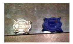
The next steps are cleaning up the casting, adding prongs to the piece to hold the stone in. add a tube to the back to hold the cord, pre polish, polish, add the center stone, and lastly attach the pearls.
