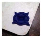
To sand-cast the piece, I filled one half of my frame with sand and tamped it down to compress the sand into a cohesive block. Next I placed the model in the sand and attached the upper half of the frame. I filled that with sand and tamped it down to make sure every depression of the model was filled with sand.. Very carefully I removed the two halves, removed my model that ended up
